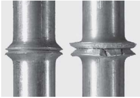
Fig. 2 Without upsetting specimen (left) and complete welding process specimen (right)
